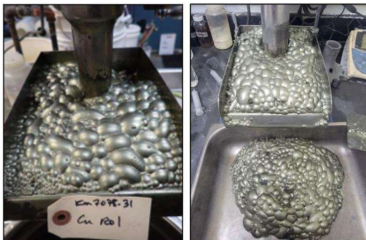
Laboratory testing of copper flotation
