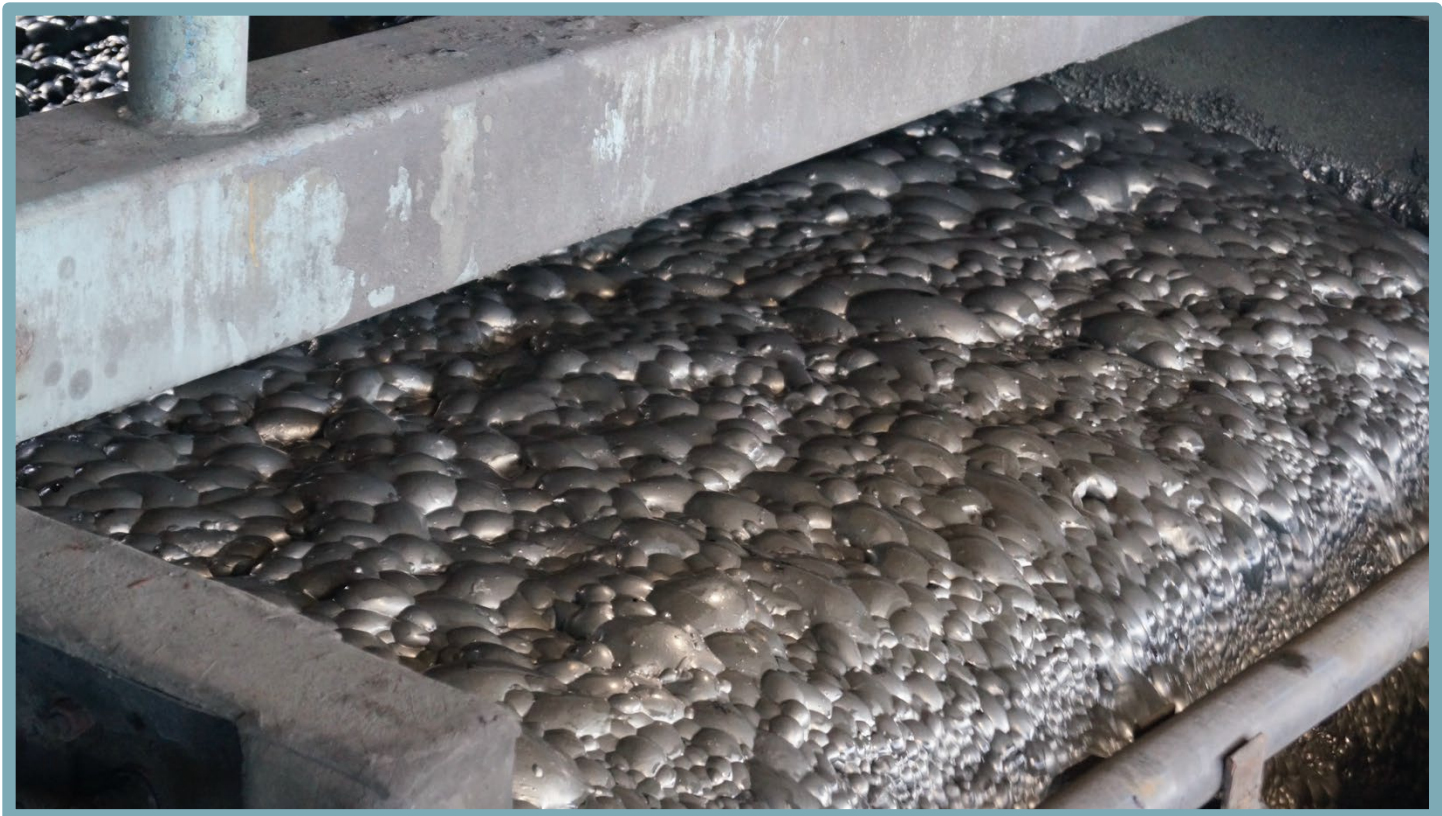
Zinc flotation cell at Campo Morado
